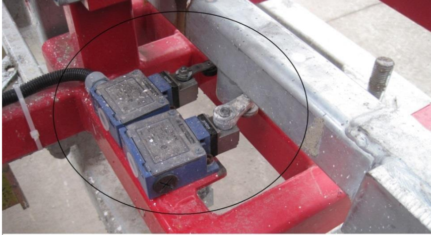
The area marked in the picture above, 2 PCs. Switch. Works by these switches trigger handle scales.
